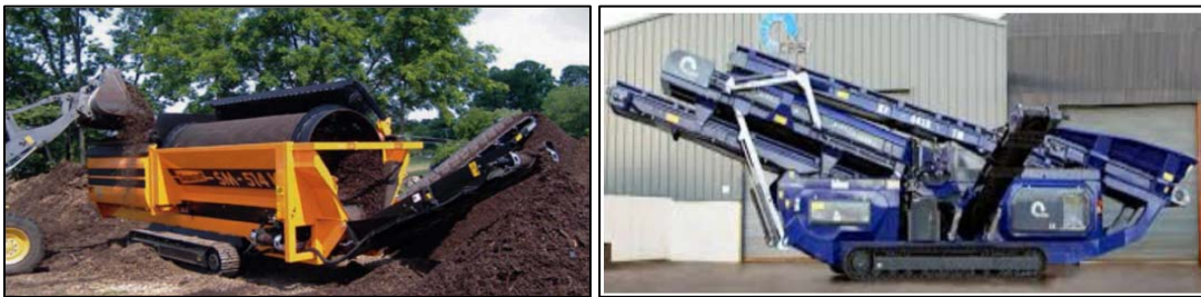
2. Proposed mechanical trommel and screener
